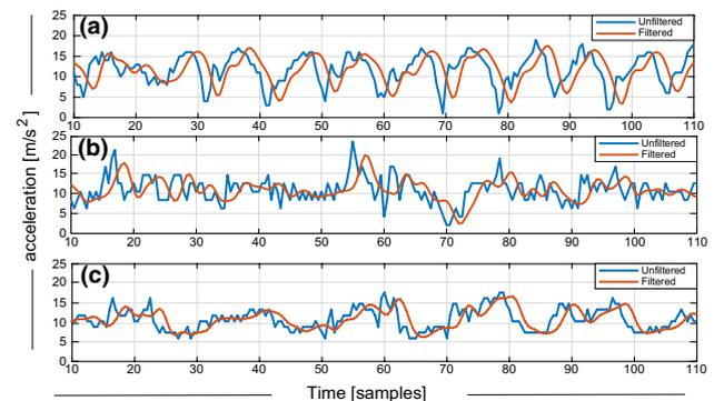
Fig. 2 Triaxial ( $x, y, z$ ) accelerometer signal of walking activity having **a**  $x$  signal component **b**  $y$  signal component, and **c**  $z$  signal component, respectively
