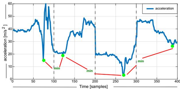
Fig. 5 Min signal feature applied over brush teeth activity sequence
